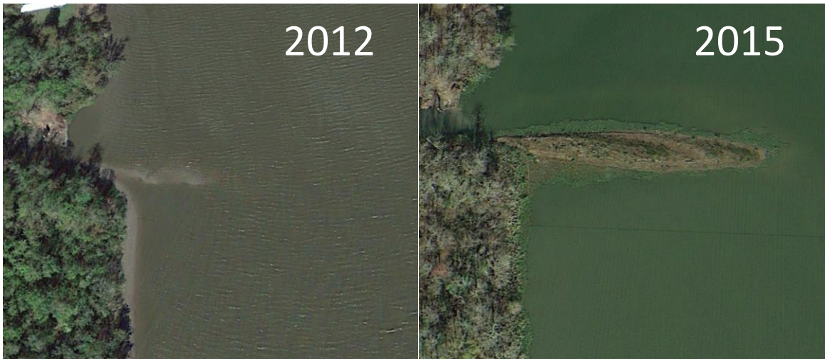
Figure 1: A 2011 breach of an Atchafalaya River channel training feature has caused rapid habitat degradation and navigational hazards in Grand Lake.
